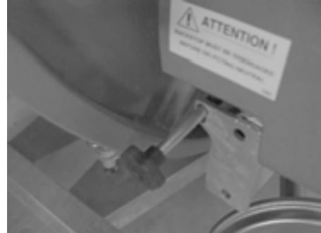
2. Drum anti-reverse engage and disengage lever.
