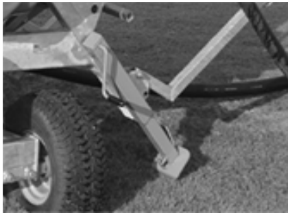
3. Mechanical crank-down anchors
