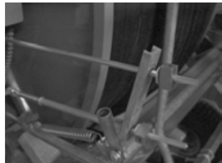
6. Automatic disengage linkage rods for shut off valve and gearbox.
