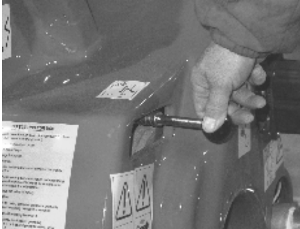
1. Gearbox engage and disengage handle
