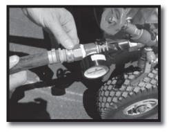
MPORTANT: MAKE SURE SUPPLY HOSE IS CLEAN AND FREE OF FOREIGN OBJECTS THAT WOULD PLUG THE TURBINE SYSTEM OR SHUT OFF VALVE! INLET CONNECTION IS FITTED WITH A DEBRIS STRAINER THAT MAY NEED TO BE CHECKED FROM TIME TO TIME AND CLEANED IF FOREIGN OBJECTS OR MATERIAL ARE PRESENT IN INCOMING WATER.
