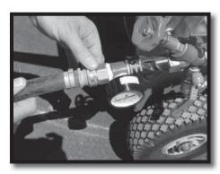
10) Once the speed is set, the MR25 will automatically roll the tube on the drum and stop at the end of the run utilizing the shut off valve.
