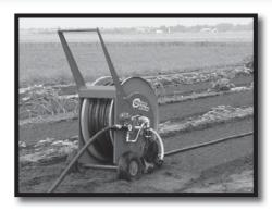
Push the machine to the desired location. Position the machine with the sprinkler cart facing the direction to be irrigated. Insure that the machine is sitting level in order for the tube to wrap properly.
