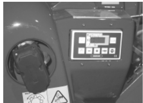
6. Electric motor regulates by-pass when using the optional computer system
